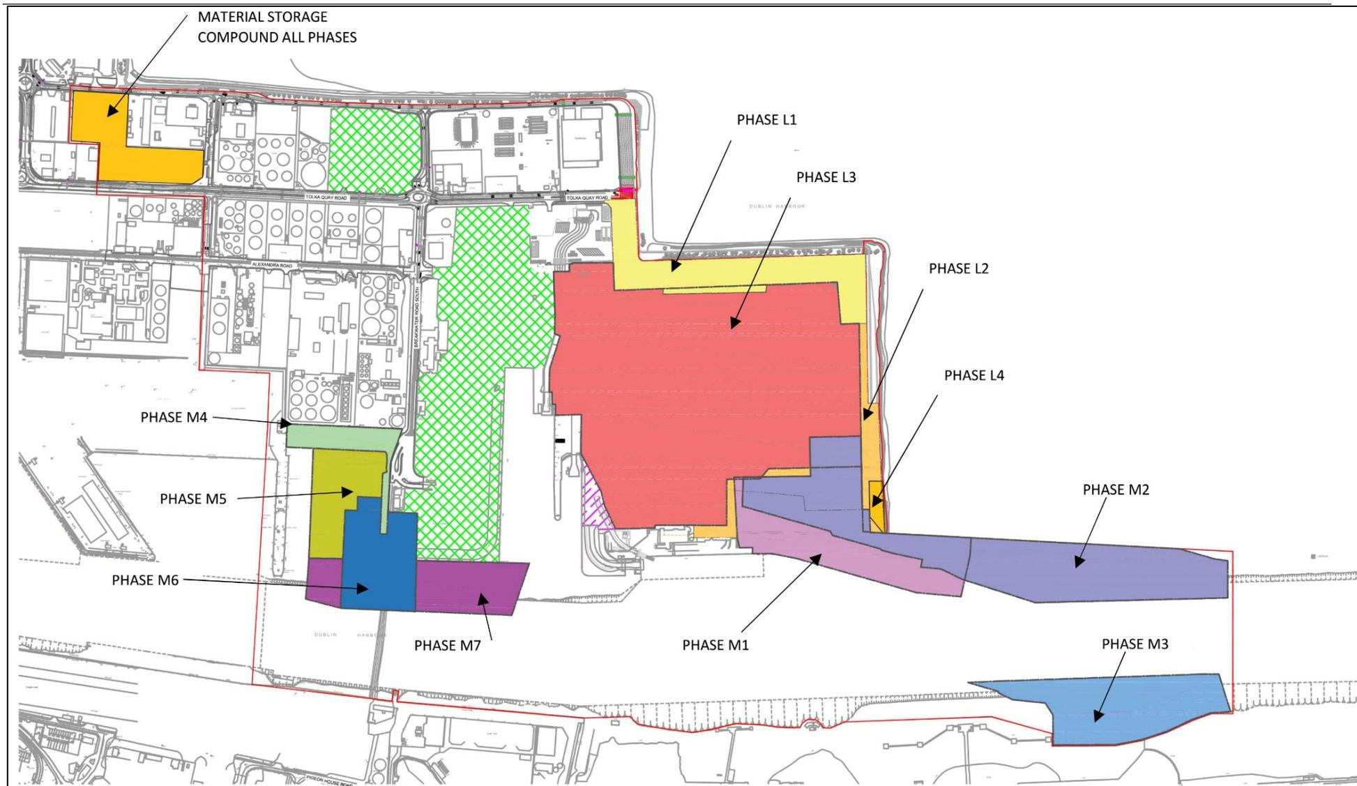
Figure 3-14 Plan of general project phasing
